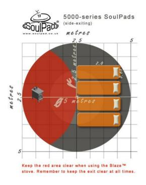
In all cases where the Blaze-flue is used, the stove needs to be sited away from the centre of the SoulPad, closer to the 'wall', with the flue pipe fitted through the canvas 'roof' via the silicone collar included with the Blaze-flue kit.
