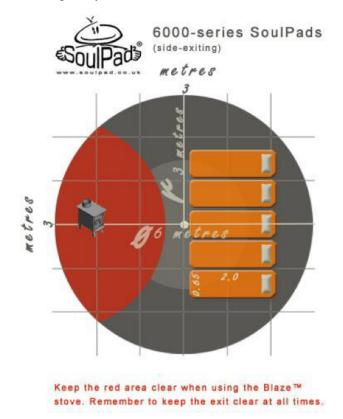
In all cases where the Blaze-flue is used, the stove needs to be sited away from the centre of the SoulPad, closer to the 'wall', with the flue pipe fitted through the 'roof' via the silicone collar included with the Blaze-flue kit.
